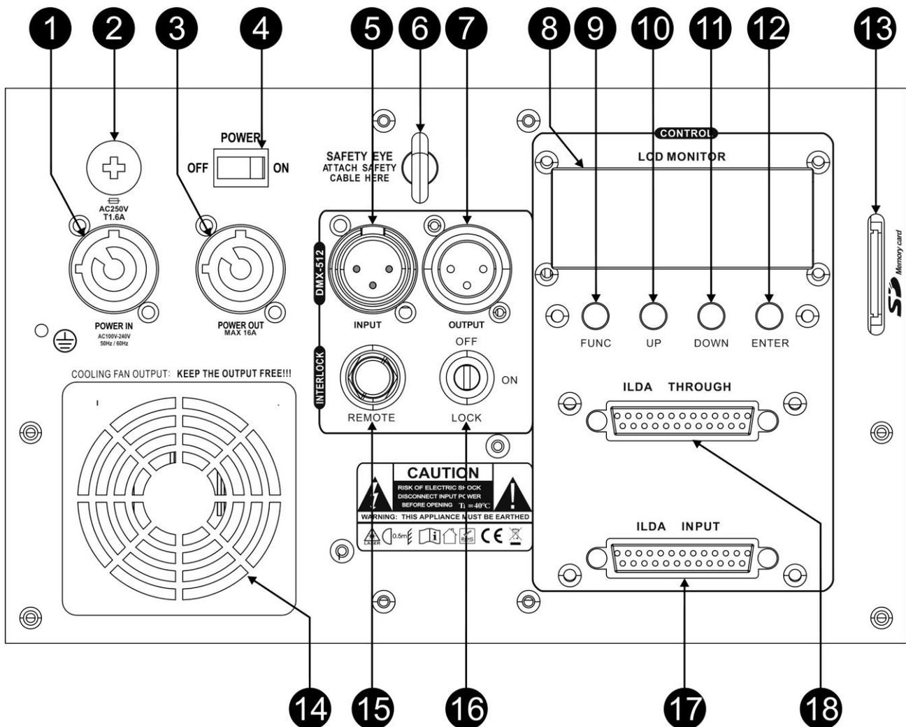
1. **[POWER IN]:** connect the supplied mains cable here.
